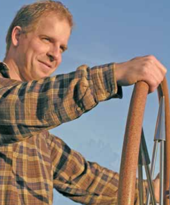
18 Yacht steering wheel of polished stainless steel, with TWIN spokes and reinforced outside ring of compressed cork
