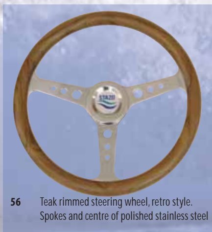
50 Teak rimmed steering wheel, retro style. Spokes and centre of polished stainless steel
